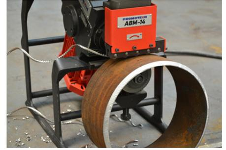
Oval workpiece and pipe beveling
